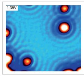
Scanning tunneling spectroscopy map of an EuO film on top of graphene. The color scale represents the local density of states at E=1.35 eV. Circular standing wave interference patterns of electrons scattered at point defects are visible. Scan size 10.3 nm × 8.8 nm, imaged at 5.3 K.
